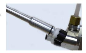
If the valve is locked, insert a 4mm Allen wrench on the back of the tool, place the assembly on the valve and loosen.
