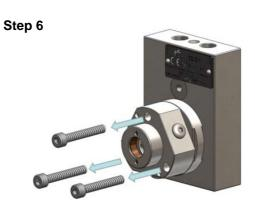
Remove the sealing unit (6).
