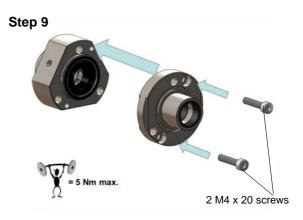
Place a new O-ring on the sealing unit.
