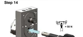
Install a new O-ring on the pump body.
