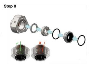
Screw the sealing unit body on the cover.
